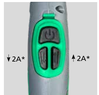
Up/Down module with 3-function key for adjustment of welding current. The welding current is increased / reduced with 2 amps. Long press for constant increase / decrease. 80300064
