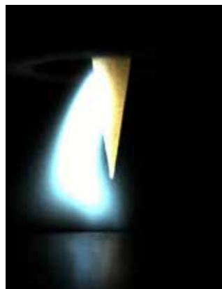
Low-quality tungsten: typically sideways arc ignition, the arc flashes and wanders slowly to the electrode tip which has to be cut off and reground.
